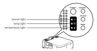
If the projector is not working correctly, first turn it off and unplug it. Then plug the power cord back in and turn on the projector. If this does not solve the problem, check the status lights on top of the projector and try the solutions recommended below.
