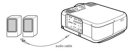
2. Connect the RCA plugs to the speaker or PA system. Insert the cable's red plug into the Audio R jack, and the white plug into the Audio L jack of the external speaker system.
