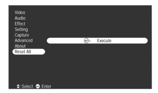
Select Reset AII and press the Enter button on the control button or remote control to display the confirmation screen. Select Yes to reset all the default settings or No to cancel.
