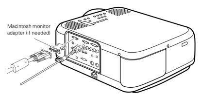
5. Tighten the screws on the connectors.
