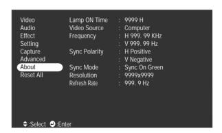
The life span of the lamp is about 1500 hours. If the number shown is close to 1500, make sure you have a spare lamp handy.
