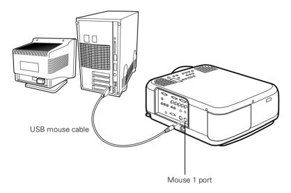
2. Disconnect your Macintosh's mouse cable. Connect the other end of the projector's mouse cable to the mouse or USB port on your Macintosh.
