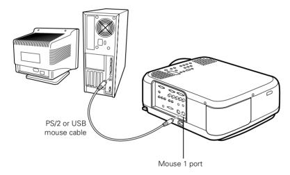
2. Disconnect your mouse from the port on the back of your computer and replace it with the other end of the cable. (Your computer's mouse will be disabled while you are using the remote control as a mouse.)
