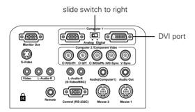
Using the tip of a pen or a small screwdriver, slide the Computer 1 interface switch to the right. (If you need to use the projector's analog port again, be sure to slide the switch back to the left.)
