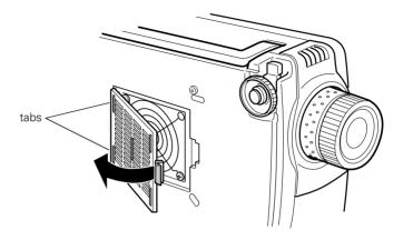
5. To install the new filter, first insert the tabs, then press on the catch until it clicks in place.
