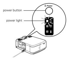
The power light flashes green as the projector warms up, and the projection lamp comes on in about 30 seconds. The power light stays green, and you may see a blue screen with the message No Signal displayed. This is normal.
