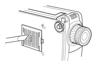
If the dirt is difficult to remove or if the filter is torn, replace it. Contact your dealer or call EPSON at (800) 873-7766 in the United States and Canada to obtain a new one.
